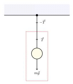
Figure 7.2: Tension in a rope. There are opposite and equal forces at either end of the rope.
