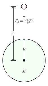
Figure 6.6: Consider a particle of mass m at a distance r from the centre of a planet of mass M and radius R that is escaping to infinity.
