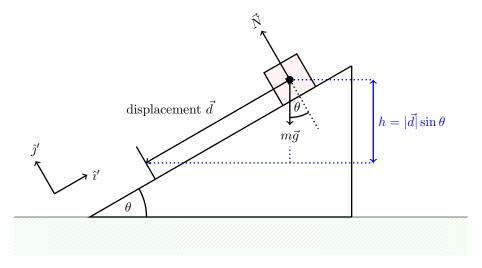
Figure 6.2: A block of mass m sliding down a frictionless plane.
