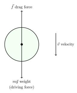
Figure 5.17: Drag force  $\vec{f}$  acting on a sphere falling through a fluid due to gravitational force  $m\vec{g}$ . The velocity of the ball is  $\vec{v}$ .
