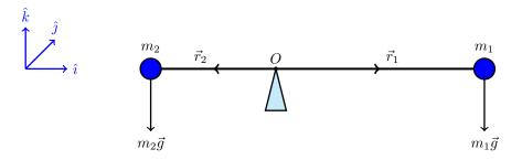
Figure 8.8: A system "balanced" so there is no net torque about the origin.
