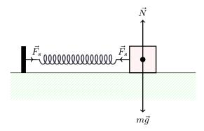
Figure 5.13: A block on a horizontal, smooth table attached to a spring.
