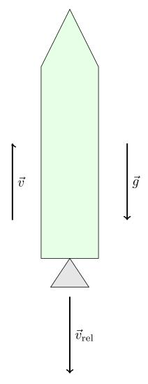
Figure 5.4: Rocket heading upwards showing the relative directions of the rocket velocity, exhaust velocity, and gravity.
