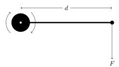
Figure 13.5: A spanner of length d and a force F acting perpendicular to the spanner.
