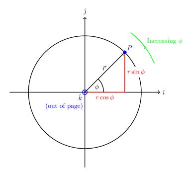
Figure 8.5: Circular motion of particle P. The angle  $\phi = \omega t$ . The coordinates of P are (x,y) or  $(r,\phi)$ .
