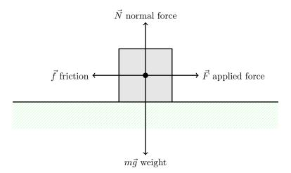
Figure 5.14: A block on a table subject to an applied force and friction opposing its motion.
