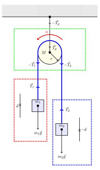
Figure 8.14: An Atwood machine with a massive pulley.
