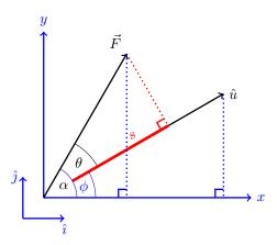
Figure 5.7: We can then find an expression for this projection using the components of the vectors in a particular coordinate system.
