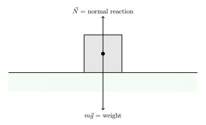
Figure 5.9: A static block at rest on a table.
