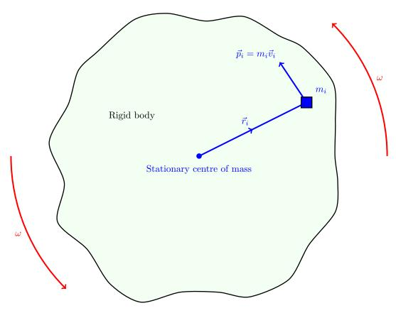
Figure 8.12: Rotational kinetic energy can be found by summing the kinetic energies of N individual elements, each of mass  $m_i$  and momentum  $\vec{p}_i$ .
