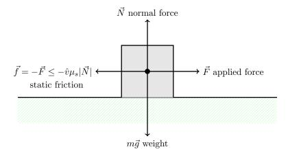
Figure 5.16: Static friction for a block on a rough table that is being pushed, but is not moving.
