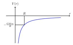
Figure 6.9: A plot of the gravitational potential V(r) as a function of r.
