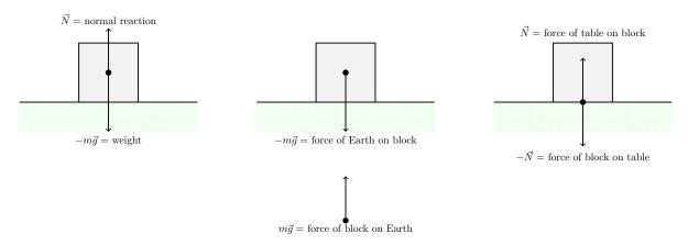
Figure 7.1: Normal reaction force between a block and table. The diagram shows the forces acting on the block and identifies the correct Newton's third law pairs.
