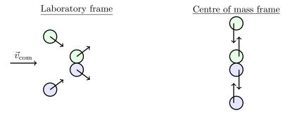
Figure 6.11: A 2D problem in the laboratory frame (left) can be transformed into a 1D problem in the centre of mass (com) frame (right). This is much simpler to solve.
