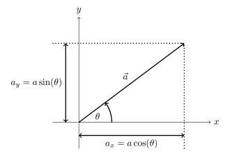
Figure 3.3: Components of a two dimensional vector a are obtained by projecting the vector onto the x-axis and y-axis.
