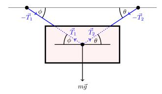
Figure 5.10: A static picture hanging form two wires.
