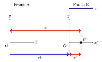
Figure 4.1: Galilean transformations between two inertial (i.e., not accelerating) frames A (with unprimed coordinates) and B (with primed coordinates).
