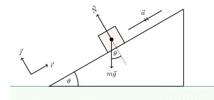
Figure 5.12: A block on an inclined smooth plane. The forces are not balanced so the block has an acceleration  $\vec{a}$ .
