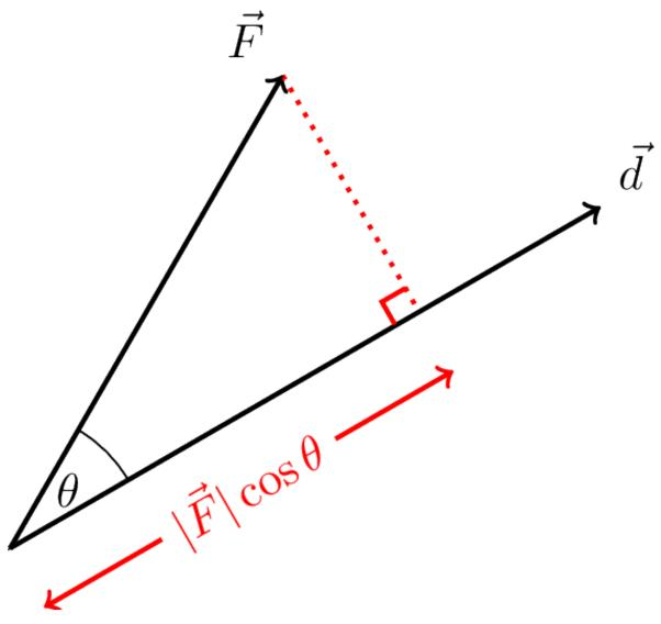
Figure 6.1: Work done, W, by a force  $\vec{F}$  at an angle  $\theta$  to the displacement  $\vec{d}$  is given by  $W = |\vec{F}| |\vec{d}| \cos \theta = \vec{F} \cdot \vec{d}$ .
