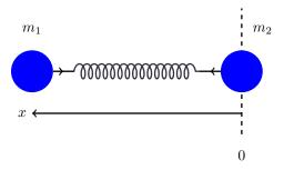
Figure 7.7: Two beads attached by a spring. We'll analyse this motion from a frame in which  $m_2$  is at rest (this is *not* an inertial frame because it is accelerating).
