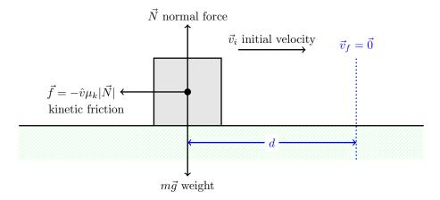
Figure 6.4: A block of mass m sliding along a rough surface being brought to rest by kinetic friction.
