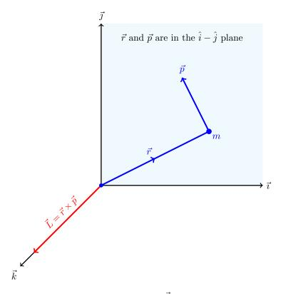
Figure 8.10: The angular momentum is defined to be  $\vec{L} = \vec{r} \times \vec{p}$  where  $\vec{p}$  is the linear momentum.
