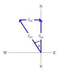
Figure 3.5: The desired direction is shown by the velocity of the plane relative to the ground,  $\vec{v}_{\rm pg}$ . The velocity of the air relative to the ground is  $\vec{v}_{\rm ag}$ , and the velocity of the plane relative to the air is  $\vec{v}_{\rm pa}$ .
