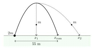
Figure 4.3: A projectile of mass 2m is launched from the origin. At its highest point it explodes into two pieces of equal mass. One piece falls vertically while the other continues to move horizontally.
