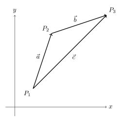
Figure 3.1: A particle moves from point  $P_1$  to point  $P_2$ , with a displacement given by the vector  $\vec{a}$ . The particle then moves to point  $P_3$ , with a displacement given by the vector  $\vec{b}$ . The overall resultant displacement from  $P_1$  to  $P_3$  is given by the vector  $\vec{c} = \vec{a} + \vec{b}$ .
