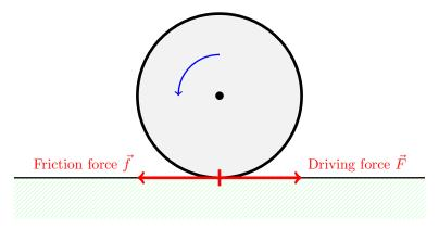
Figure 7.3: Bicycle wheel turning anti-clockwise. The wheel exerts a force  $\vec{F}$  against the road, and the road exerts a friction force  $\vec{F}$  against the wheel.
