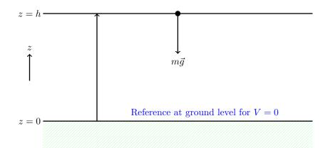
Figure 6.5: A particle of mass m being lifted through a height h against gravity. We are free to set the zero point for the potential at ground level for convenience.
