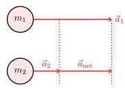
Figure 7.6: The net acceleration measured in the frame of particle 2 is  $\vec{a}_{\rm net} = \vec{a}_1 - \vec{a}_2$ . Note that because particle 2 is accelerating this is not an inertial frame.
