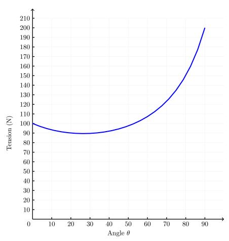
Figure 15.3: Tension in rope as a function of angle,  $\theta$ , above the horizontal.
