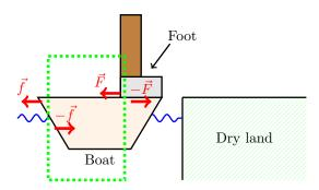
Figure 7.4: Stepping off a boat. Foot pushes against boat with force  $\vec{F}$ ; boat pushes back with force  $-\vec{F}$ . Boat pushes against water with force  $\vec{f}$  and water pushes back against boat with force  $-\vec{f}$ . The forces acting on the boat are shown in the green box.
