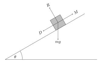
Figure 13.1: Force diagram for part (a), constant speed uphill.
