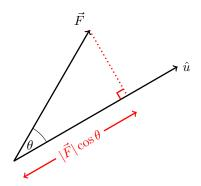
Figure 5.6: Projection of a vector  $\vec{F}$  in the direction of unit vector  $\hat{u}$ .
