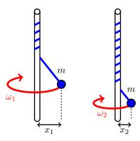
Figure 8.11: As mass m on a rope wraps around a pole its horizontal distance from the pole decreases from  $r_1$  to  $r_2$ .
