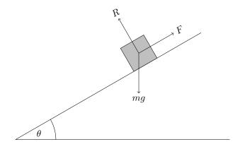
Figure 13.3: Force diagram for part (c), stationary car.
