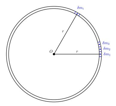
Figure 8.9: Moment of inertia of a circular ring of radius r and total mass M. The ring can be broken up into individual pieces of mass  $\delta m_i$ .
