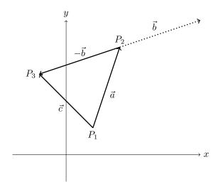
Figure 3.2: Vector subtraction. In this case  $\vec{c} = \vec{a} - \vec{b}$ .
