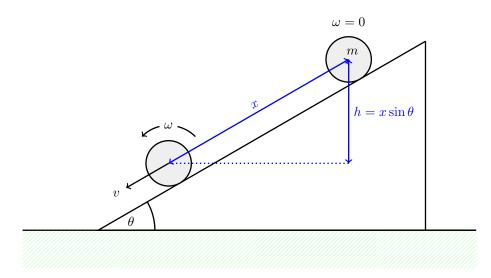
Figure 8.15: A cylinder rolling down a slope without slipping.
