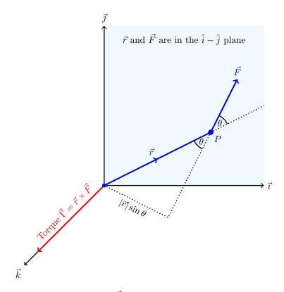
Figure 8.6: Torque produced by a force  $\vec{F}$  acting at position  $\vec{r}$ . In this diagram the vectors  $\vec{r}$  and  $\vec{F}$  are in the  $\hat{\imath}$ - $\hat{\jmath}$  plane. The perpendicular distance from the origin to the line of the force is labelled  $|\vec{r}|\sin\theta$ . The torque in this case is in the direction of the  $\hat{k}$  axis and is  $\vec{\Gamma} = \vec{r} \times \vec{F}$ .
