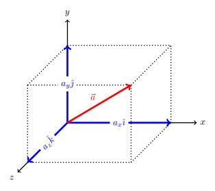
Figure 3.4: Components of a vector  $\vec{a}$  in a three dimensional cartesian coordinate system.
