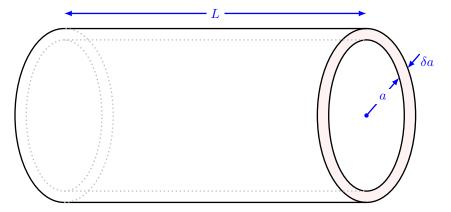
Figure 11.2: Thin cylindrical shell of inner radius a and thickness  $\delta a$ .
