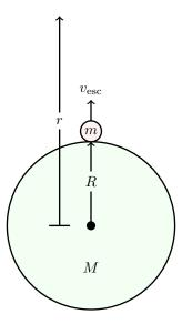
Figure 6.8: A particle of mass m with initial velocity  $v_{\rm esc}$  at a distance R from the centre of a planet of mass M that has just enough kinetic energy to escape to infinity.
