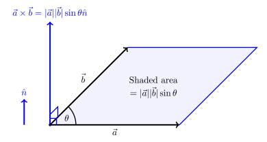
Figure 8.1: Geometrical interpretation of the cross product of two vectors  $\vec{a}$  and  $\vec{b}$ . The cross product  $\vec{a} \times \vec{b}$  has a magnitude equal to the area of the parallelogram defined by the two vectors, and is in a direction perpendicular to the plane of those vectors, in a right-handed sense.
