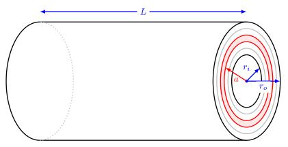
Figure 11.3: Cylindrical shells making up a thick cylinder of inner radius  $r_i$  and outer radius  $r_o$ . Each individual shell (shaded in red) has a moment of inertia given in part (a).
