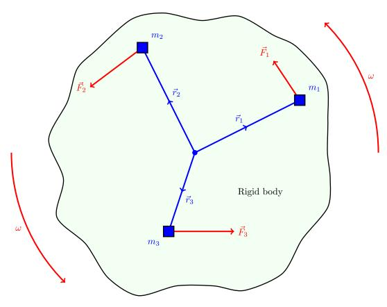
Figure 8.7: Torque on a rigid body made up of N individual masses,  $m_1, m_2, \ldots$  at positions  $\vec{r}_1, \vec{r}_2, \ldots$  acted upon by forces  $\vec{F}_1, \vec{F}_2, \ldots$  The origin is placed at the centre of rotation, which need not be the centre of mass. Because this is a rigid body there is one common angular velocity ,  $\omega$ . The figure only shows three of these masses for clarity.
