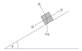
Figure 13.2: Force diagram for part (b), constant speed downhill.
