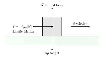
Figure 5.15: Kinetic friction for a block sliding along a rough table.
