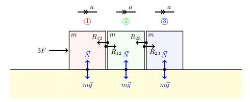
Figure 7.8: Row of three blocks in contact with one another. The left-most block is being pushed by a force 3F.
